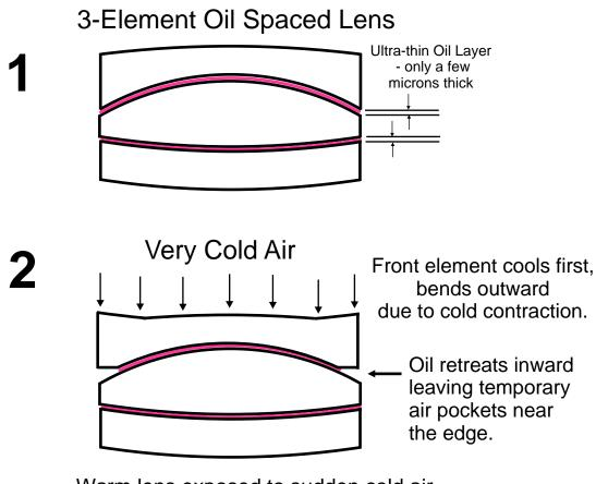
Warm lens exposed to sudden cold air conditions when taken from a warm room directly into a freezing night air.
