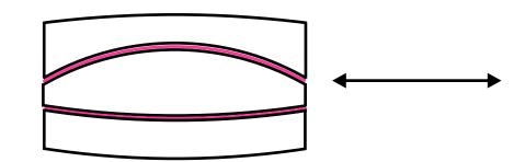
After a period of time, the entire lens cools to outdoor ambient temperature. The elements settle back to their normal shape and the oil migrates back to the edges. The lens is now settled down.
