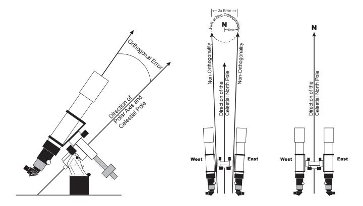
Traditionally, correcting orthogonality (sometimes called "cone error") involves meridian delays and flipping back and forth across the meridian to observe how far from image center that the star falls. This is time consuming and involves trying to remember whether you need to advance or delay the flip time in order to swap sides. Is it east side or west side?...advance or delay?...groan!
