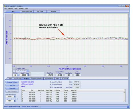
4. Once you have loaded this curve into the controller's memory (CP1 thru CP4), you can now turn on PEM and do one more run of 1 to 3 worm cycles to see how well the mount now tracks.
