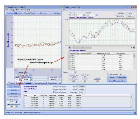
2. Next step is to create a PE curve from this data. Press the button to create new PE curve. A new window will pop up which shows a basic fitted curve with the major harmonics and their values.
