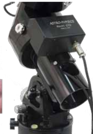
3. Pull short cable leg through and connect to R.A. Servo Drive
