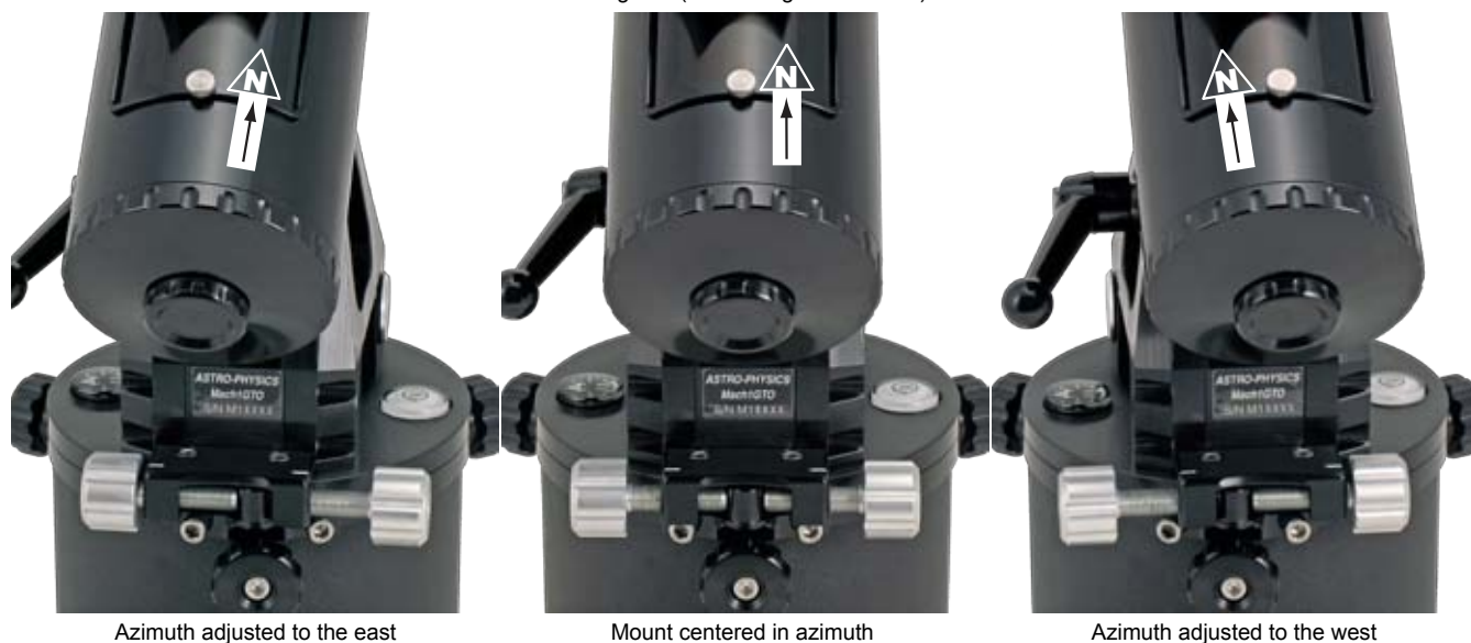
Mach1GTO Azimuth Adjustment Range 13 degrees (+/- 6.5 deg. from center)
