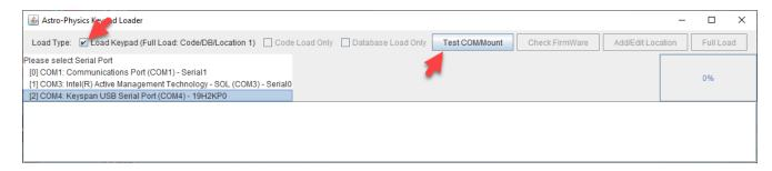
6. Click Test/COM Mount button. Results should display as follows:
