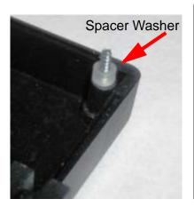
Be careful not to lose the six spacer washers. Some may stick to the circuit board instead of staying on the screws. It is best to place the spacers onto the screws right away. This will keep you from losing them, and it makes lining things up easier on re-assembly.
