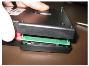
The cable strain relief may need to be held and guided gently into the cutout in the case to finish mating the two halves.
