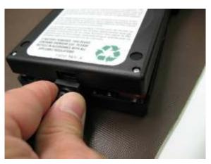
Make a final check to be sure that no wires, fibers or cables are caught between the front and back halves of the keypad.
