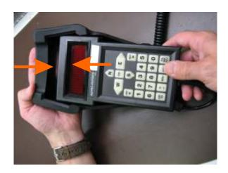
Finally, work the cable the rest of the way through and carefully stretch the thin part at the bottom of the KEYPRO over the cable's strain relief. (See instructions from p.1.) Again, be very careful that you neither tear the thin part of the KEYPRO, nor do any damage to the strain relief.
