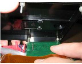
13. When placing the back on the unit, first be sure that all six spacers are in place on the screws. Then, make sure the screws are aligned with the proper holes. Start by aligning the two screws on one side of the display. Make sure that all wires fibers and cables will be safely inside the unit. Line up the display end before moving to the cable end of the keypad.
