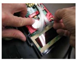
Guide the lithium battery wires under the fiber-optic cable and plug it into the battery connector. The black lead is normally to the outside.
