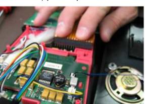
Plug the display cable into the display header making sure the pins are aligned
