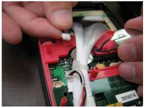
8. To completely remove the lithium battery: CAREFULLY guide the lithium battery wires under the fiber-optic cable as shown in the next few pictures . . .
