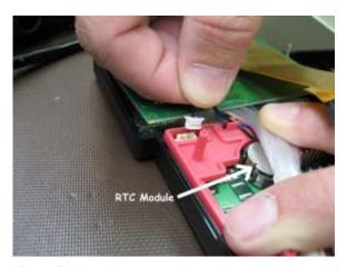
View of lithium battery cable connector unplugged
