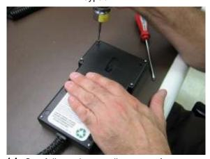
14. Carefully apply a small amount of pressure to hold the back down while tightening all six screws to 2-2.5 in-lbs (torque).
