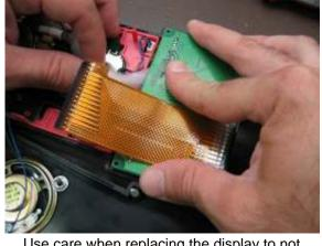
Use care when replacing the display to not scratch the window or to damage any of the optical fibers. Carefully place the display in the front of the case
