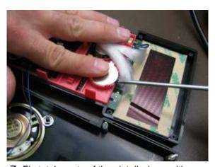
7. First, take note of the pigtail wire positions relative to the sides of the battery holder so that you orient the new battery correctly. Carefully remove the battery from the battery holder as shown with your small flat blade screwdriver.
