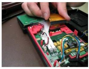
View of display connector unplugged. At this point, the display can be carefully removed from the keypad. Lay the display aside on a soft surface. Be very careful not to scratch the glass on the front of the display.
