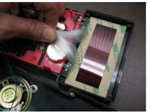
11. Gently pull the fiber-optic cable away from the window before replacing the display. You do not want to crush or sharply bend any of the fibers.
