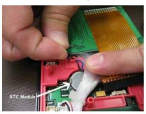
6. Remove lithium battery wires from the red plastic spacer's molded clamp.
