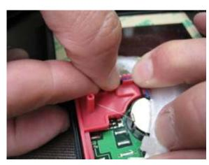
10. Snap the battery wires into position by pushing them into the spacer's molded clamp. Be careful not to catch any fiber-optic cables!
