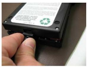
The cable strain relief may need to be held and guided gently into the cutout in the case to finish mating the two halves.
