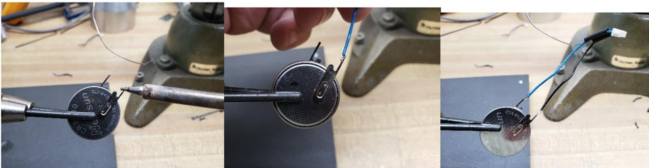
6. After cooling, slide the heat shrink back down the wire and press it onto the tab. You can use the soldering iron to gently warm and shrink the tubing down on the connection, but a heat gun will work better.
