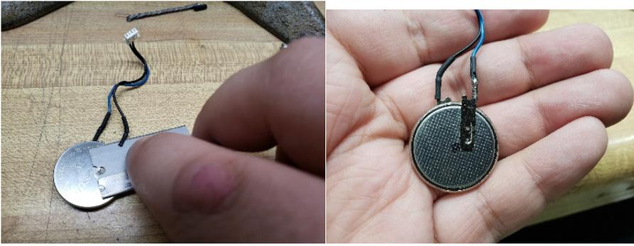
3. Use the soldering iron to quickly heat the soldered joints, and pull the wire away from the tab. This should be quick as to not burn the heat sensitive insulation on the wires.
