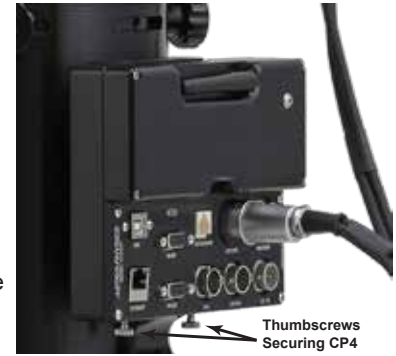
Mach1GTO with CP4 Attached to Pier
