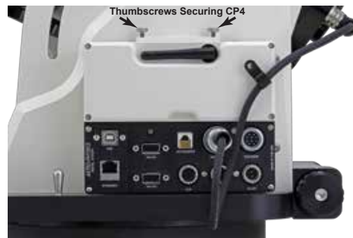
1600GTO and 3600GTO Style with CP4 Attached to Polar Fork 1600GTO shown
