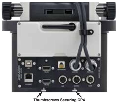
1100GTO and 1100GTO-AE/L with CP4 Attached to Mount Base
