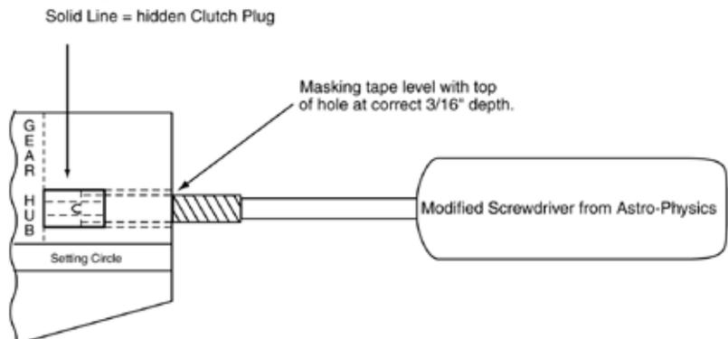
cause the old clutch plug to be “unscrewed” from the clutch hole. You may need to use considerable turning force at first to get the old plug to start to “unscrew” itself.
