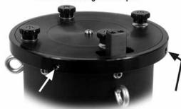
Attach to an Astro-Physics pier. Simply fit the Rotating Pier Adapter into your Astro-Physics Portable Pier just like the Standard Pier Adapter (900SPA) and fasten it from the side with the six screws and washers provided. Make sure that the Azimuth Adjuster Block is on the north side.
