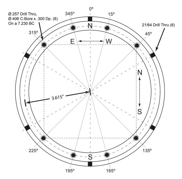
The drawing above provides the necessary detail to drill and tap your flat surface to accept the 900FSA Flat Surface Adapter for 900 mounts (all versions). The eight counter-bored 1/4"-20 thru-holes are all on a 7.230" bolt circle (3.615" radius).
