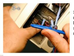
Step 47 - There is no need to press the motor spur gears tight against each other before applying final torque to the screws. Light finger pressure is all that is required. (3-e)
