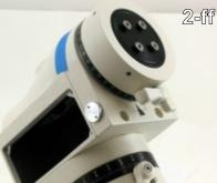
Step 39 Return the finished declination shaft assembly to the declination/motor housing. (2-ee, 2-ff)
