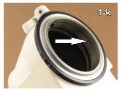
Step 7 - The exposed plain-bearing surface machined into the aluminum casting is used in manual rotation. Wipe clean and grease with Lubriplate No 105. (1-k)
