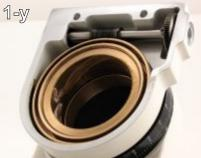
Step 14 - When you are ready to reassemble, put the worm wheel back in the housing if not already there. Don't forget the brass ring! Place the worm housing onto the wheel as shown, fully engaging the teeth. (1-x,1-y)
