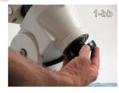
Step 17 - Return the pre-load ring to the rear of the RA shaft and rotate it until it makes contact with the rear bearing. Then, back it off approximately 1/8 turn or 15-20 degrees. Lock down all 3 screws as evenly as you can. (1-bb)
