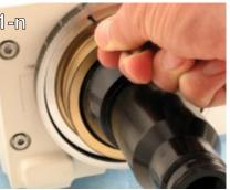
Step 8A -Since the right-ascension circle retaining ring is exposed, this is a good time to check that it has not backed off. Simply insert your 2mm hex key into one of the two holes provided and use it to rotate the retaining ring clockwise until tight. (1-m, 1-n)
