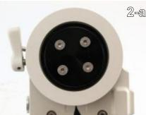
Step 18 - Since you have disassembled everything, you will need to align the worm housing so that it is squared up with the declination/motor housing. Apply some pressure to the worm and lock down the two mounting screws. With no motors in place, adjust the tightness by placing your hand into the housing and rotating the right ascension worm spur with your fingertip. Once no backlash is present and the spur gear turns with your finger, you are done. (1-cc, 1-dd)
