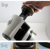
Step 27 - Push up from the bottom, (counterweight side) to remove the declination shaft and worm wheel from the housing. (2-o, 2-p)
