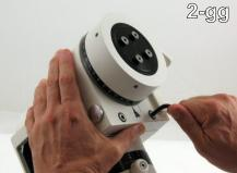
Step 40 Push the worm housing up against the worm wheel and put the two M6 SHCS and washers back into place. Tighten lightly. (2-gg)
