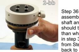
Step 36 - To check that you have assembled this part correctly, hold the shaft and rotate the worm wheel gear. It should turn easily with a little more drag than when the gear was first put in place in step 32. If not, back off the 4 screws from Step 35 and re-tighten evenly or go back to step 34 and back off the pressure on the ring. (2-bb)
