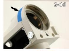
Step 38 Engage the right-ascension clutch knob to keep this axis from moving. Place the worm housing on the declination/motor housing. Use some painters masking tape to keep in place if you like, but don't put any screws in yet. (2-dd)
