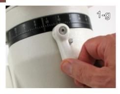
Step 5 - Release the tension on the clutch knob. It is not necessary to undo any of the screws in the knob.(1-g)
