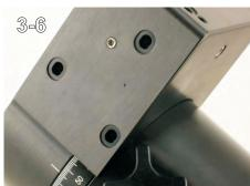
Remove the five worm drive retaining screws from each side of the mount. (3-5, 3-6, 3-7) Use a 3/32 inch hex key.
