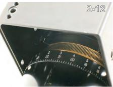
Remove the worm drive assembly completely from the right-ascension housing. (2-11, 2-12)
