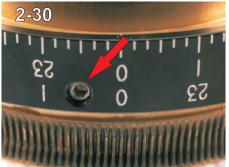
The worm wheel acts as a plain bearing for the shaft in manual movement of the mount and needs to be removed for cleaning and greasing. You must remove the gear by grabbing it directly. Do not lift by the R. A. setting circle as the grease suction between the gear and shaft is stronger than the spring and ball (2-31) that holds the circle in place under the set screw seen in 2-30. (2-29)
