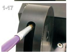
Lubricate the tip of the altitude rod if not already done as well as the pocket it rotates in. (1-16, 1-17)
