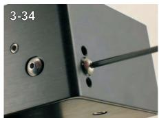
Next insert the two long set screws. You will adjust the position of the screws to remove backlash a little later. (3-35)
