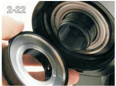
With the screws backed off sufficiently, completely remove the knob. (2-21, 2-22)
