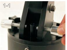
Back both azimuth screws out and clear of the azimuth pin. (1-1)
