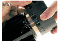
Grab the end of the shaft assembly and pull the shaft and worm wheel straight out of the housing. (2-26, 2-27, 2-28)
