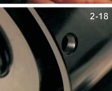
The right-ascension end shaft knob has to be removed next. A hole is provided in the housing to allow access to the set screws in the knob. (2-18)
