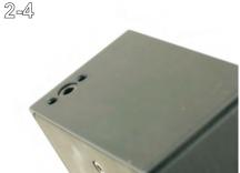
Start the right-ascension housing disassembly with the removal of the three push pull screws. Use a 3/32 hex key. (2-3, 2-4)
