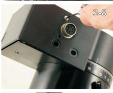
Remove the two screws retaining the receptacle. (3-8)
