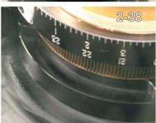
Place the worm wheel back on the shaft and push it all the way down to a firm stop. Rotate several times to distribute the grease and confirm that it is down. (2-37, 2-38)
