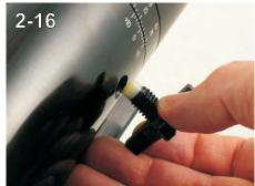
Remove both clutch knobs. There is a Delrin plug between the knob and the worm wheel gear it mates with. It can stick to the knob as it comes out or may hang up inside. It can usually be captured by touching the tip of the knob to it. (2-15, 2-16, 2-17)
