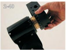
Place the shaft assembly back into the housing. Make as certain you can that the gear enters squarely with the housing or it will seize up or lock instead of going in. (2-39, 2-40)
