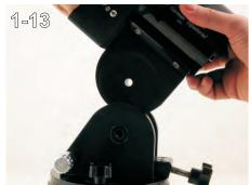
Grab the mount firmly with the clutch knobs engaged and lift it straight up out of the forks. (1-12, 1-13)
