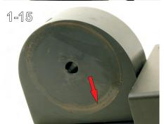
Clean and lubricate the bearing rings and the surface they engage on the center plate. (1-14, 1-15)
