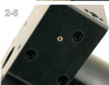
You must also remove the five button head screws retaining the worm drive. Three are on one side of the housing (2-5, 2-6) and the other two are on the opposite side near the plug receptacle. (2-7)
