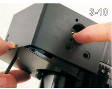
Use a flat end 9/64th hex key to break the worm drive free. Push in the receptacle to free the harness. (3-10)
