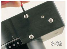
With pressure applied to the worm drive assembly, insert and lightly tighten the five drive-retaining screws. (3-31,3-32, 3-33)
