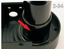
Clean and grease the inside diameter of the housing. (2-33)
