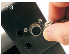
Remove the two button head screws retaining the receptacle. Use a 1/16 inch hex key. (2-8)
