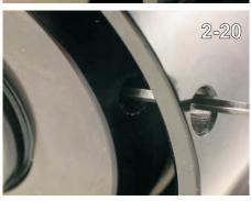
Before releasing the screws, rotate the shaft by hand so that you can feel the dampened resistance that was set at Astro-Physics. You will need to reset the mount to this same feel later.
