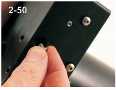
Rotate the shaft end cap until it comes to a stop and then back it off approximately 5 degrees.(2-41)
