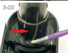
Pull the declination worm wheel from the shaft. If the gear will not pull off then use the gravity method detailed in image 2-32. (3-19)
