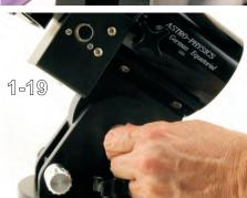
Place the mount back in the forks. It will meet the altitude rod at some point which will help you to support the weight. Line up the holes and insert the SHCS. (1-18, 1-19)
