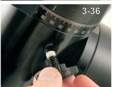
Return and tighten the two clutch knobs making certain that the Delrin tip is still in front of the knob. (3-36)
