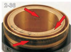
Clean and grease the outer bearing surfaces of the gear as well as the inside and face. The teeth can also be relubricated with Lubriplate No. 105. (2-35, 2-36)
