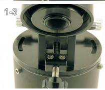
Remove the azimuth lock knobs from both sides. (1-2, 1-3)
