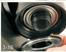
Remove the shaft end cap. (3-15, 3-16)
