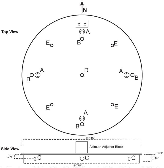
The 1200 series mount is designed to fit our 10" outside diameter pier, which is available in several heights. The pier adapter of the 1200 mount shown above fits into the post (aluminum tube) of the pier assembly and is secured with six (6) 5/16-18 screws at the location marked C.
