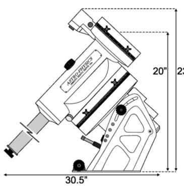
The diagram shows several dimensions that are commonly requested. In addition, if the scope is horizontal and pointing west or south, the measurement from the top of the pier to the middle of the cradle plate is 11.25." Please note that these dimensions will vary somewhat depending on your latitude. We quote them for 42 degrees because that is the latitude of Astro-Physics and all of our equipment is set up that way. It is also a good average value.
