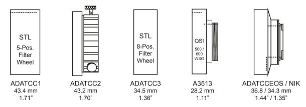
**Spacing from the rear flange (not threads) of the 175FF and 160FF with Backfocus Spacers removed.** For imaging trains that require more than the 80.8 mm backfocus spacing, the Backfocus Spacer can be removed to provide additional room for such items as off-axis guiders. The allowable spacing without the Backfocus Spacer is shown below. The drawing references the AP 130 GTX distance. The equivelant TEC scope distances are listed below.
