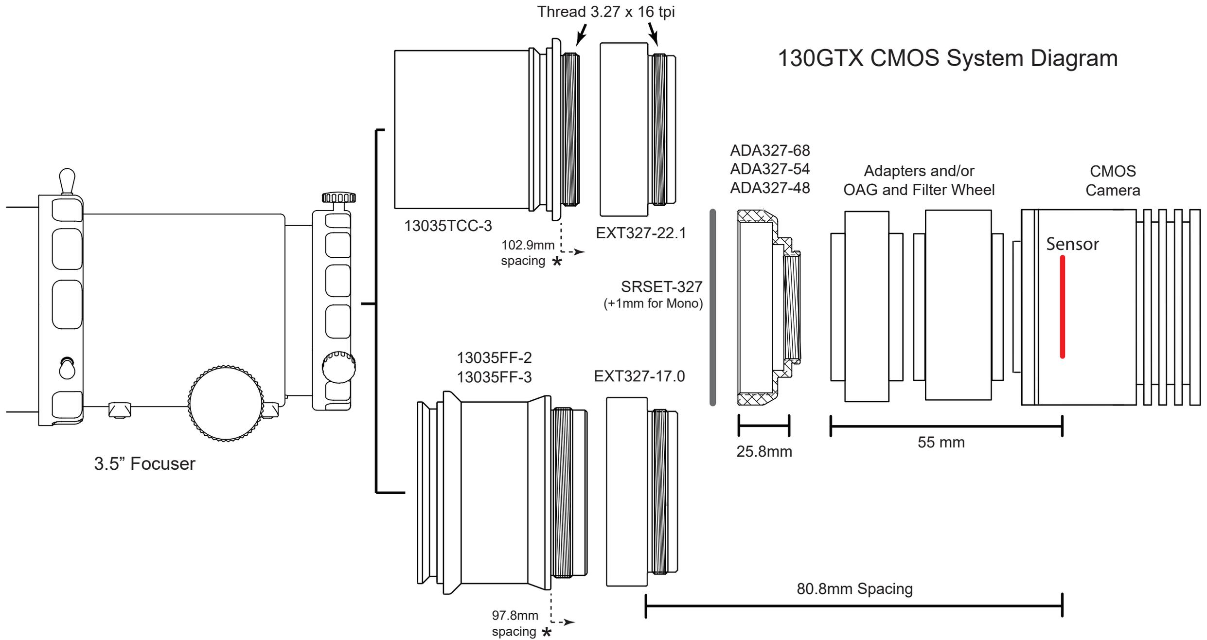
\* For specialized camera equipment that requires more than 80.8mm backfocus spacing distance you must provide your own adapter. Do not use AP adapters and extensions shown above.
