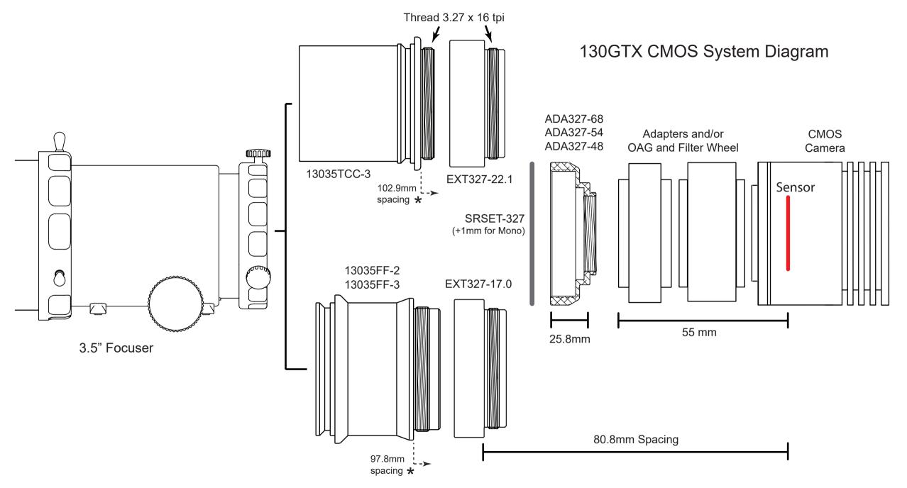
\* For specialized camera equipment that requires more than 80.8mm backfocus spacing distance you must provide your own adapter. Do not use AP adapters and extensions shown above.
