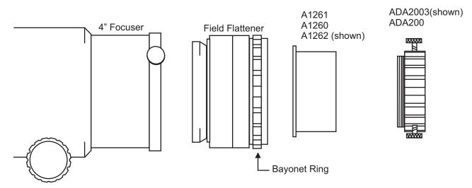
Remove the bayonet ring of the field flattener. Place the CCD adapter against the machined surface on the field flattener assembly. Thread the bayonet ring back in place, which secures the CCD adapter. The 2" adapter (ADA2003 or ADA200) will thread onto the part of the CCD adapter that extends beyond the bayonet ring. Insert your CCD camera with its 2" nosepiece (either our AP16T or nosepiece that you already have.) and you are ready to image.
