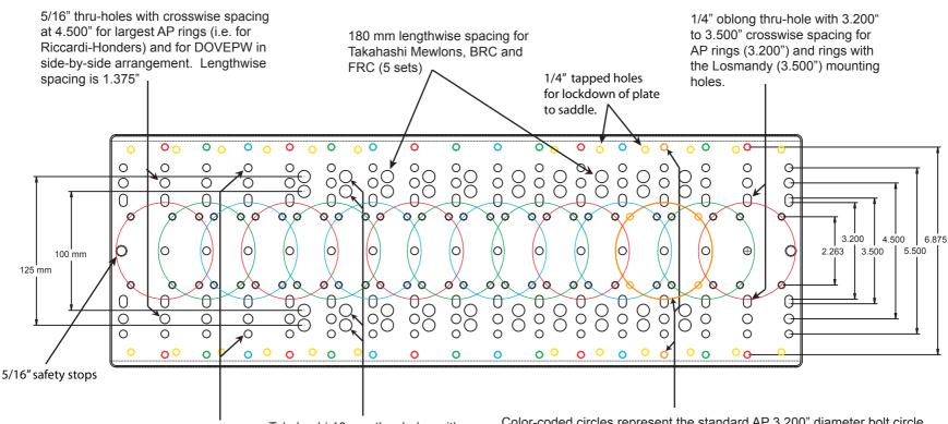
1/4" thru-holes with 5.500" crosswise spacing are available for custom applications. Lengthwise spacing is at 1.375" for the 5.5" sets.
