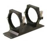
Attach the Astro-Physics 12" Sliding Bar (SBD12) to the 4.7" rings with four 1/4-20x1 1/2" flat head socket head cap screws. (Do not use the center holes.) This provides a solid 2-hole connection for each ring. Photo shows SBD12 and 47RING.
