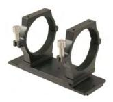
You can raise the scope another half inch above the plate by using Losmandy AP blocks (LMAPBLOCKS) between the rings and the plate. First, attach the blocks to the bottom of the rings using the supplied 1/4-20x1/2" socket head cap screws – two per ring / block assembly. Then fasten each ring / block assembly to the 12" Sliding Bar with two 1/4-20x1" low-profile socket head cap screws (4 total). Refer to the photo to see how this looks. Photo shows SBD12, LMAPBLOCKS (set of 2), 47RING.
