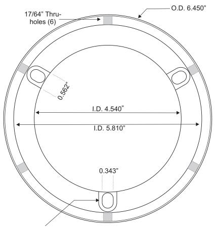
3 Slots spaced 120° apart for 5/16" or M8 Socket Cap Screws on a 5.110" bolt circle.
