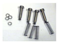
If the pinion block shoulder screws have spacers under the springs (some do, some don't), remove the springs and spacers. Keep the orientation of the springs the same as they were (do not turn them end for end).
