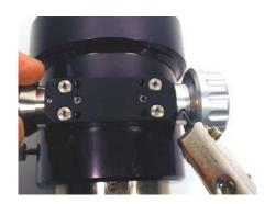
Loosen the knob opposite the reduction gear with a 5/64" (Traveler and 2.7" Focuser) or 1/16" (4" Focuser) hex key and remove it from the pinion.
