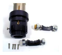
With a 3/32" hex wrench, remove the 4 screws holding the standard pinion block and knob assembly from the focuser body.
