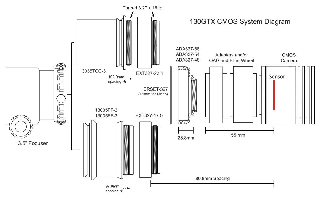
★ For specialized camera equipment that requires more than 80.8mm backfocus spacing distance you must provide your own adapter. Do not use AP adapters and extensions shown above.
